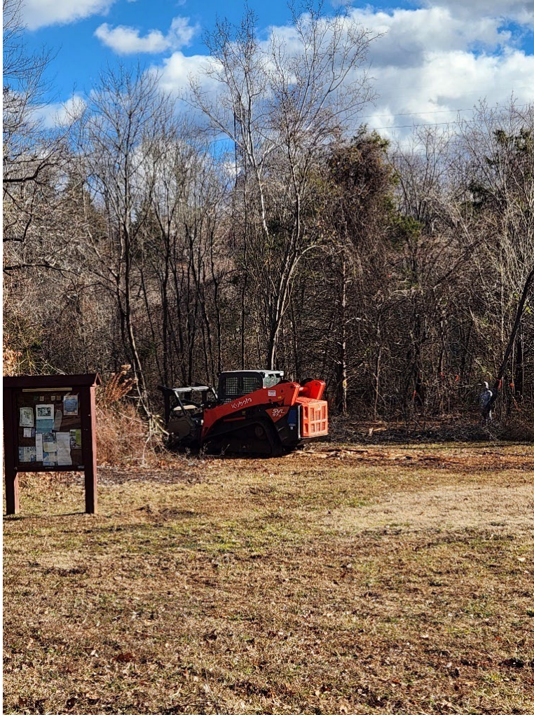
Figure 7) Forestry mulcher at Riverview Park. December 2025. (mechanical IPM practice)
